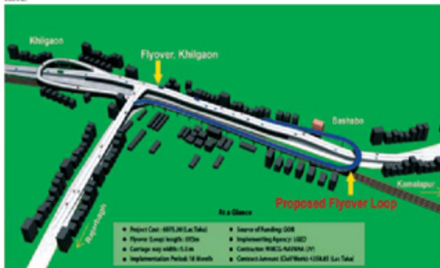
Layout plan of the loop in the Khilgaon Flyover (at Saidabad end)
