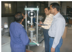
Un-confined Compression test is being carried out in the laboratory.
