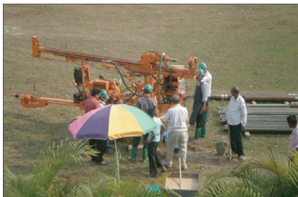
Photograph-35 : Sub-soil investigations are being carried out with Drilling Rig Machine
