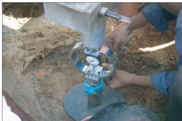
Photograph-36 : Field CBR Test is being carried out
