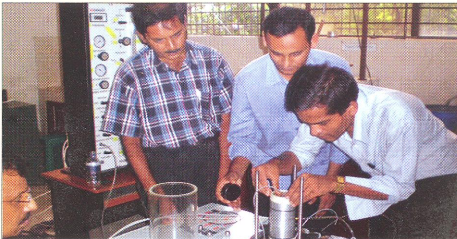
Tri-axial soil testing at the LGED Central Laboratory.
