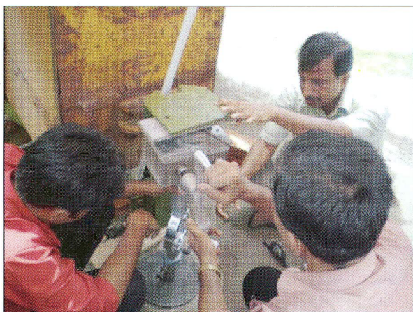
Photo 4 : Field CBR Test
