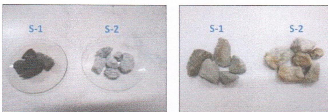
Figure 3.1: Photo images of before (left) and after (right) acid tests for both samples.
