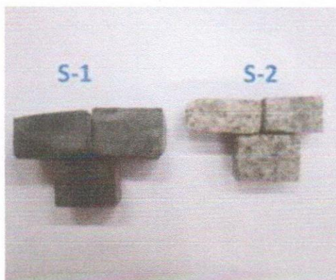
Figure 3.2: Photo images after crystallinity test. Standard method applied: ASTM C1260.
