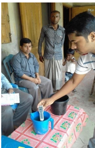
Photo 35. Picture of measurement of EC of water at Derai, Sunamganj
