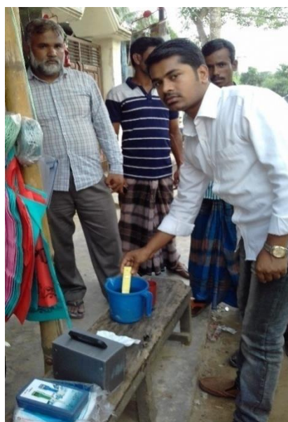
Photo 36. Picture of pH measurement with Hanna pH meter at Nasirnagar, B. Baria
