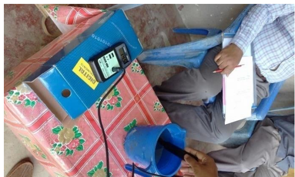
Photo 34. Picture of measurement of Dissolved Oxygen in Sadar, Sunamganj
