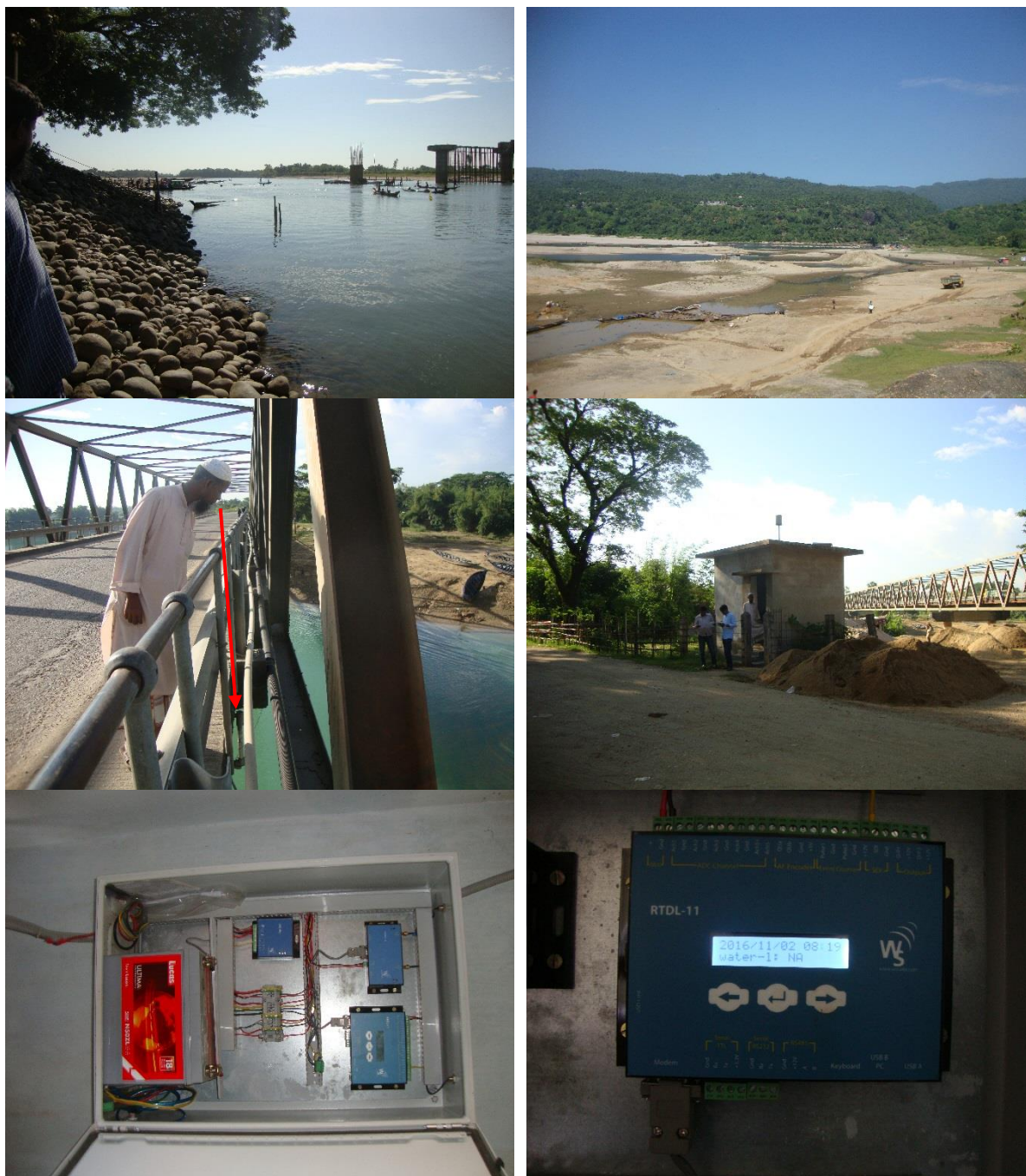
(Top) Existing manual water Level gauge at Jafflong; (Middle) Sarighat Gauge Reader is monitoring auto-gauge sensor set at the bottom of the bridge deck; (Bottom) Equipments of autogauge sensors installed inside the room
