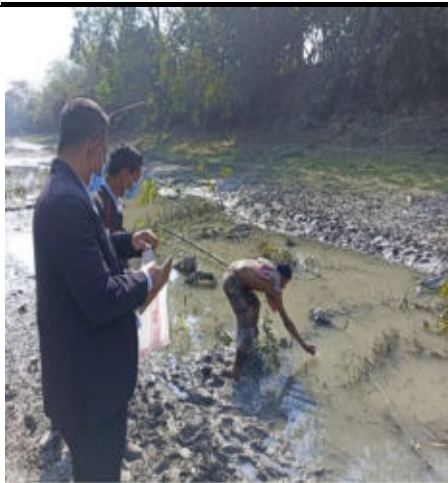
Collecting surface water sample from a nearby canal at road from Sree Rampur CRDP drain to Hawaur more bridge, Jhikorgacha/W-01(23°6'42"N and 89°6'3"E)
