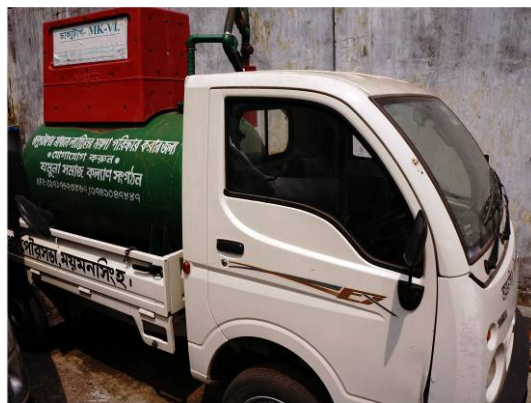
Plate 5.2: 2 cu.m capacity Vaccutug, the Vacuum tank is installed on a pick-up van
