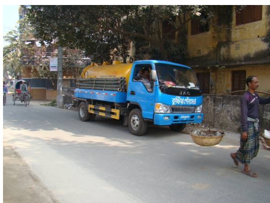
Plate 5.1: 4 cu.m capacity Vaccutug, the Vacuum tank is installed on a truck
