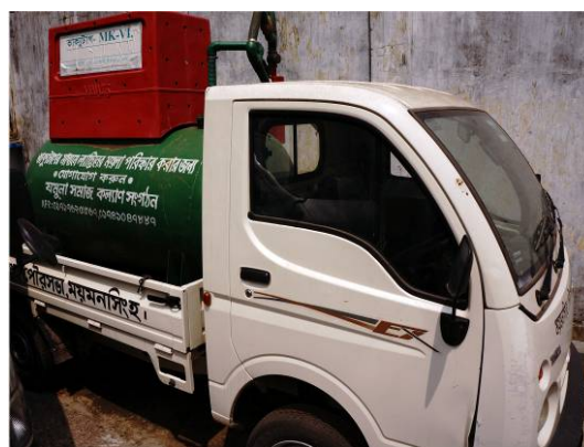
Plate 5.2: 2 cu.m capacity Vaccutug, the Vacuum tank is installed on a pick-up van
