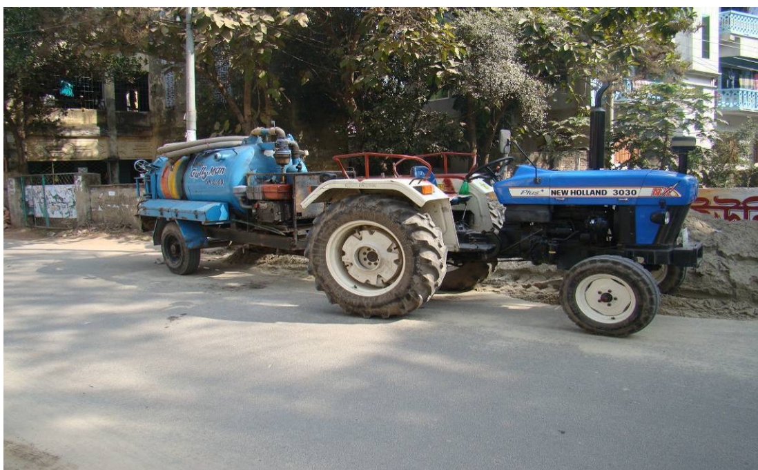
Plate 5.3: 2 cu.m capacity Vaccutug, the Vacuum tank is fixed with a tractor trolley
