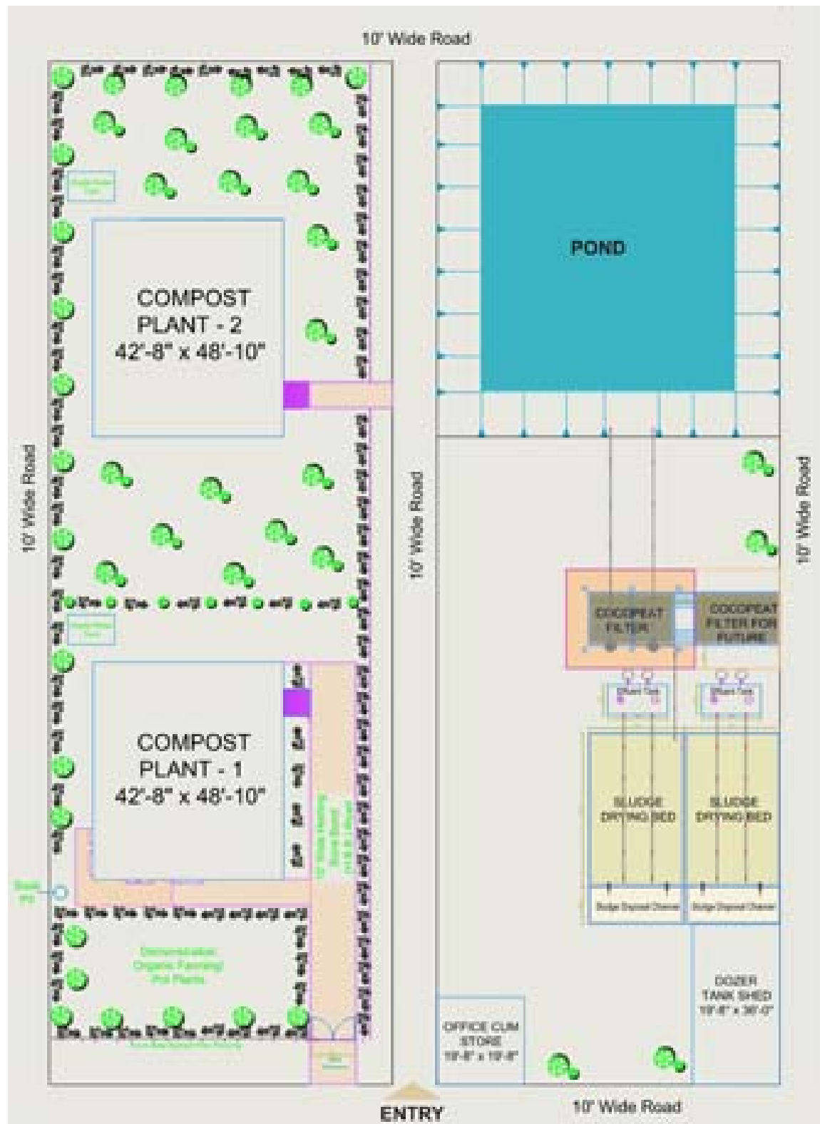
Figure A2: Site Plan of the Co-composting Facility, Kushtia
