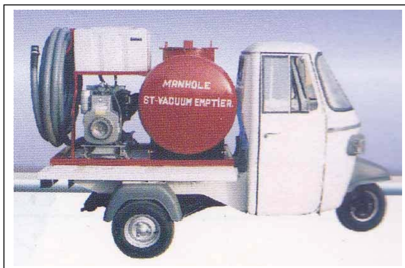
Plate 6.1: Three wheeler mounted vaccutug
