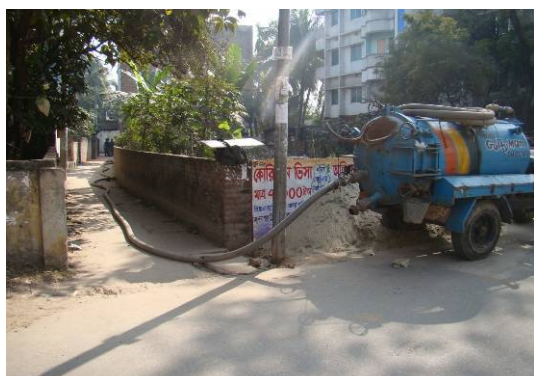
Plate A7: Vaccutug collecting faecal sludge from the households of Kushtia Municipality.
