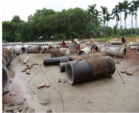
Spun concrete pipes – curing SP 31001 Rouha, Mymensingh
