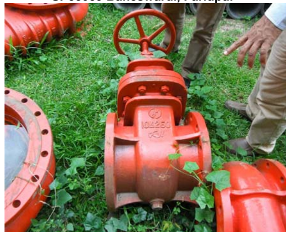
Gate valves for on / off flow control may be used instead of alfalfa valves built into flow control structures SP 41008, Goshinga, Gazipur
