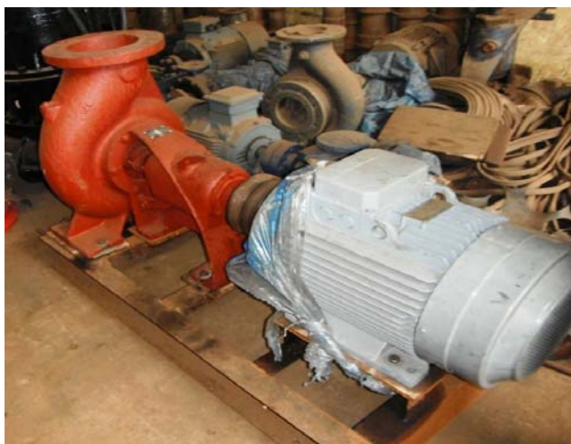
Pump set with large Milner's Pump and electric motor, Milner's Pump Factory, Tongi June 2014
