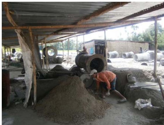
Production of Spun Concrete Pipes, Rouha
