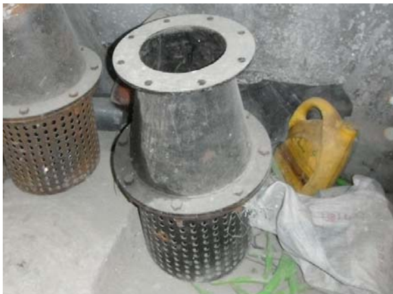
Screen and foot-valve with flange connection
