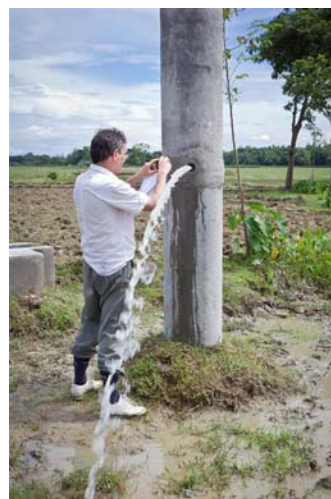
Piezometric tube not yet fixed to airvent standpipe SP 33096 Saherber Gaon, Sunamganj
