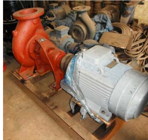
Electric motor and pump mounted on steel frame / skid, Milner Pump Foundry, Tongi, Dhaka
