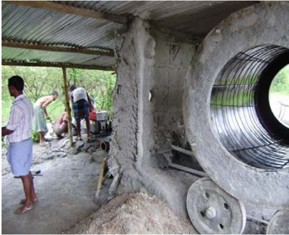
Production of spun concrete pipes (SP 31001, Rouha, Mymensingh)
