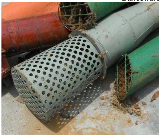
Screen (& Foot valve) at end of Suction Pipe
