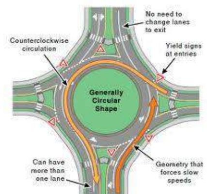
Fig 11.3: Channelization Measures at Major Intersections
