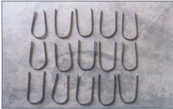
Figure 6: 'U' hook used for JGT application
