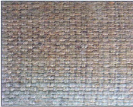
Fig 1: Bitumen treated JGT
