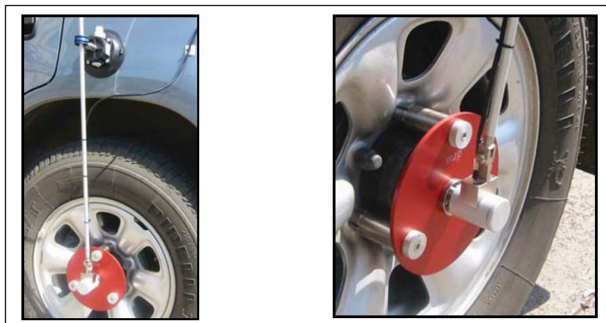
Figure 2-9 : Photo showing Rotary Wheel Encoder mounted on wheel
