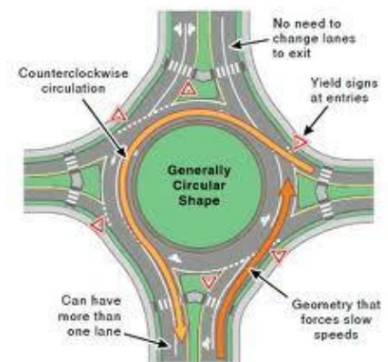
Fig 11.3: Channelization Measures at Major Intersections
