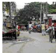
Figure 18: Carriageway encroached with park vehicle
