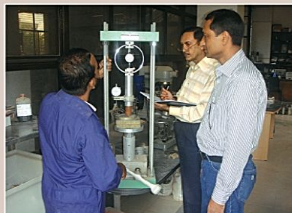
Unconfined compression test of soil sample is being processed at CQCL, Dhaka
