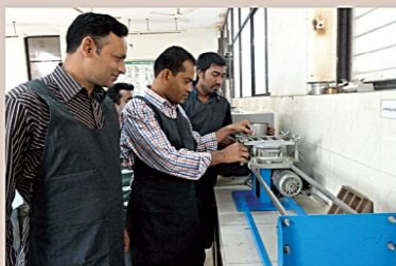
Cement cube is being compacted using Jolting apparatus (EN)
