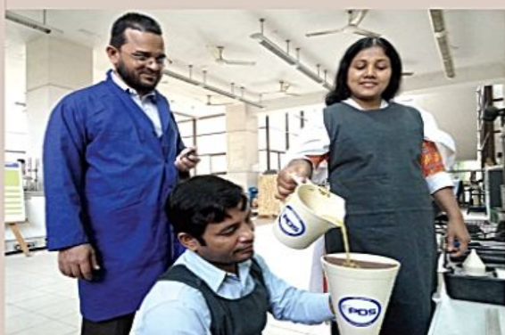
Viscosity test of Bentonite solution is in process at CQCL before allowing bentonite powder at construction site
