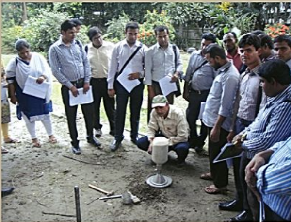
Practical Session on field density test using Sand Cone apparatus during QCT-1 course at CQCL, Dhaka
