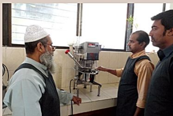
Cement mortar mixing is going on using mortar mixture for compressive strength of cement at CQCL
