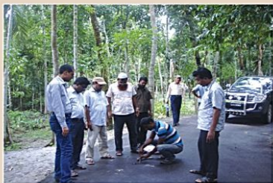
Random thickness check of bituminous layer at Bhandaria, Pirojpur by EE, CQCL
