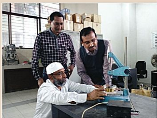
Bitumin penetration test is being conducted by LGED Engineers at CQCL, Dhaka
