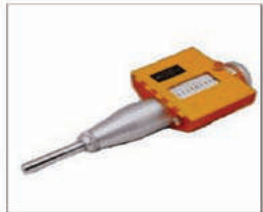
Photo-7.7.2 Schmidt rebound hammer
