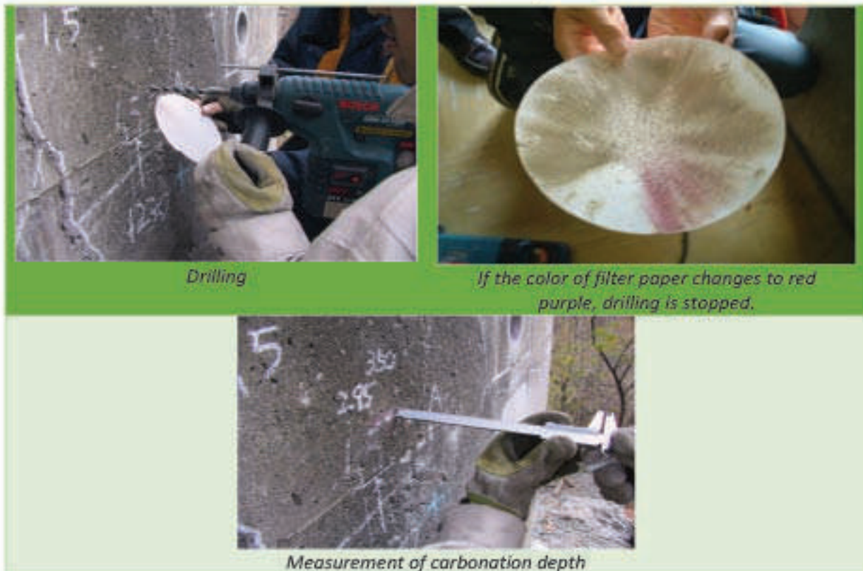
Photo-7.7.6 Phenolphthalein method by drilling
