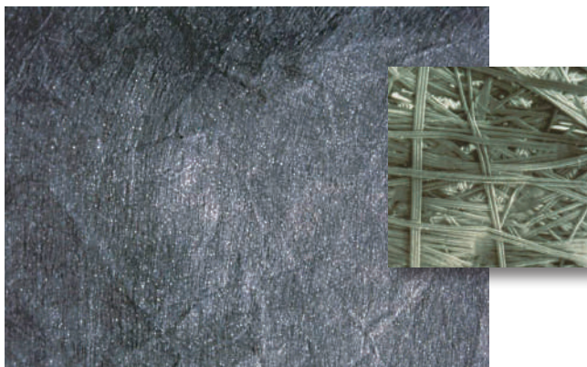
Figure 15. Non-woven heat bonded geotextile with close-up
