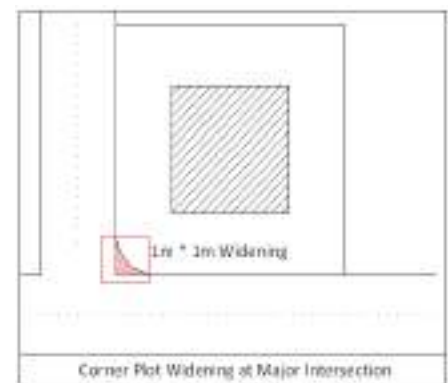
Fig 11.4: Corner Plot Widening at Intersections
