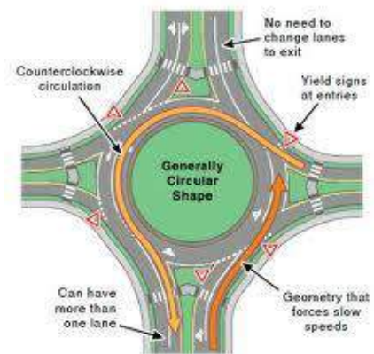
Fig 11.3: Channelization Measures at Major Intersections
